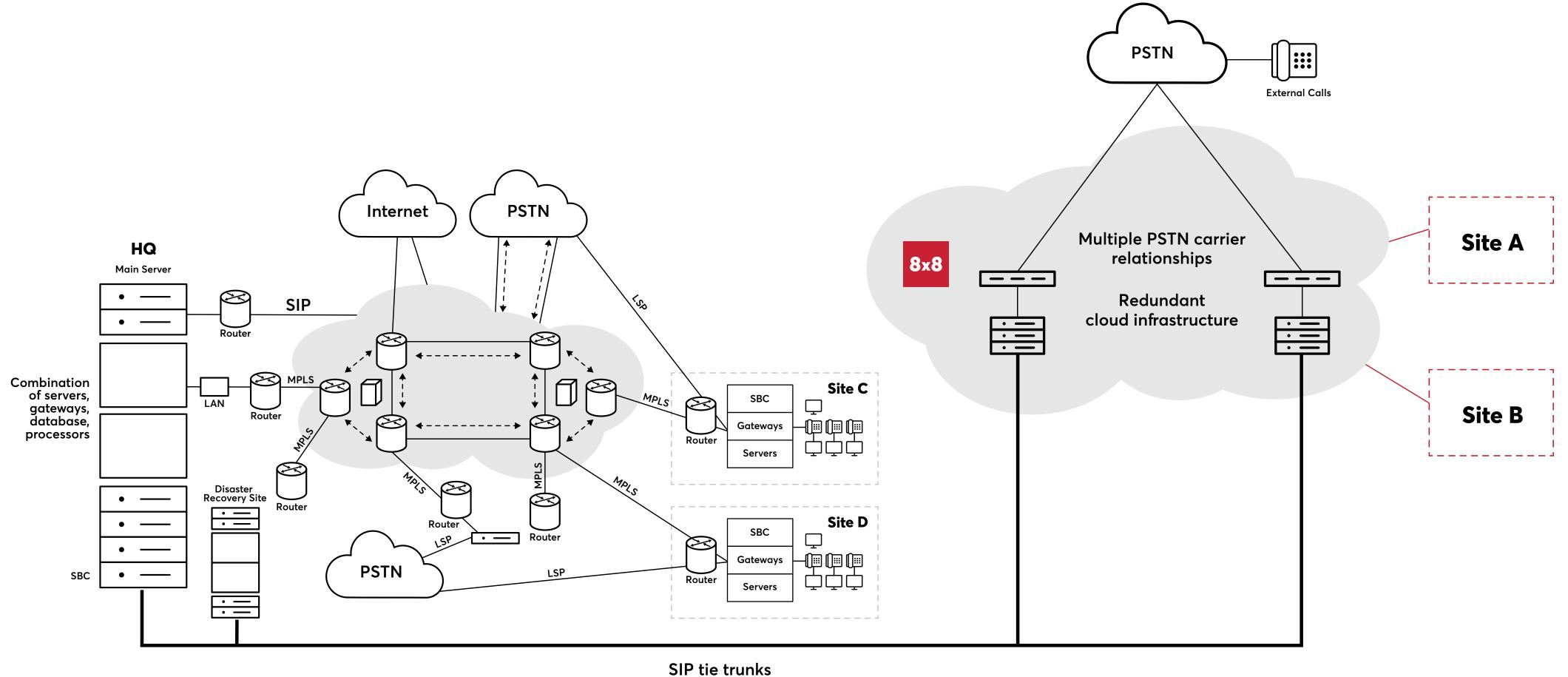
A phased, yet integrated migration can be accomplished by overlaying dial plans between the legacy footprint and the cloud, and utilizing SIP tie trunks or call forwarding to enable each set of users to seamlessly reach the other, as if it were one system across the board.
